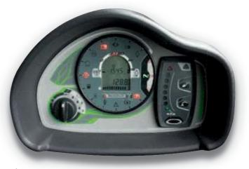
Your **safety** is further enhanced by the operater **presence detector** located in the seat. Travel movements are only allowed when you are sitting in the driving seat.
